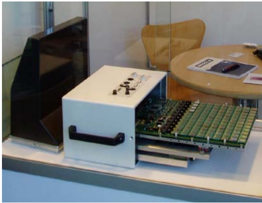
Fig. 9. Side view of the Dear-Mama detector box open with the carbon cover next to it.
