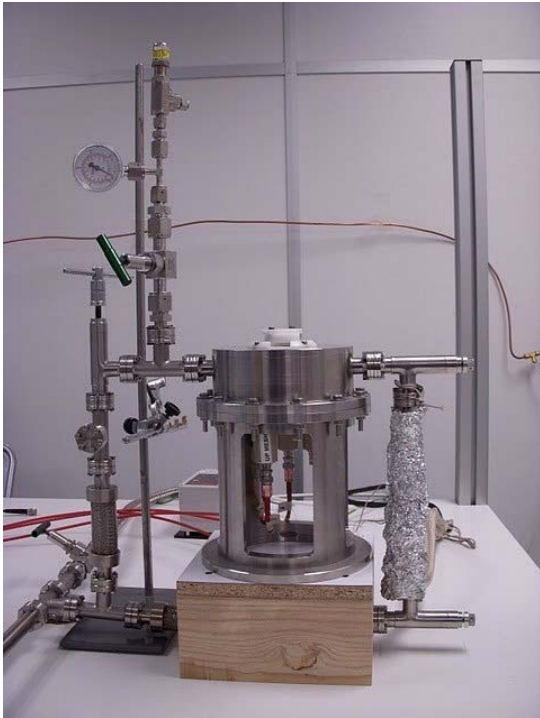
Fig.7. The NEXT R&D chamber in the IFAE laboratory, with gas piping and purification getters. The chamber can host up to five APDs.
