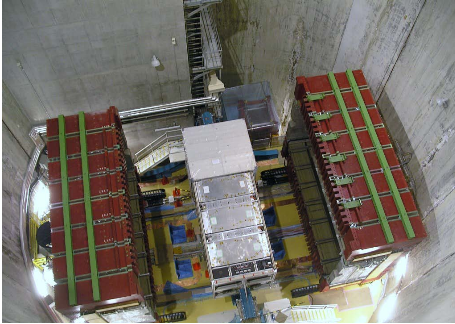
Fig. 2. View of the T2K near detector with the magnet (in red) opened so the inner detectors can be seen (aluminum boxes).
