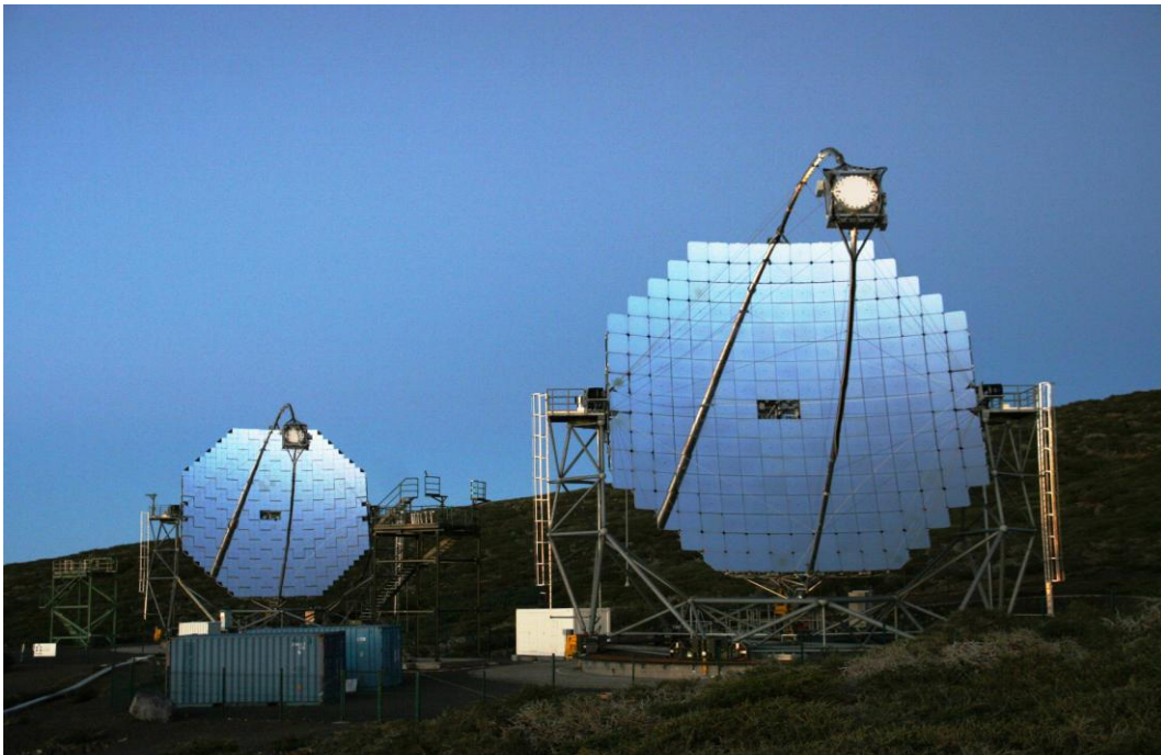
Fig. 1: The MAGIC telescope system preparing for observations at dawn. From left to right: MAGIC-I and MAGIC-II. Thanks to their large mirrors, the MAGIC telescopes working in stereoscopic mode are able to detect gamma rays of energies between \sim 50 GeV and \sim 50 TeV. They are powerful eyes to observe the most violent phenomena: the non-thermal Universe. Credit: MAGIC Collaboration.
