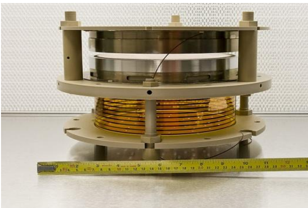
Fig. 8: Time Projection Chamber with electroluminescence detection built at IFAE.
