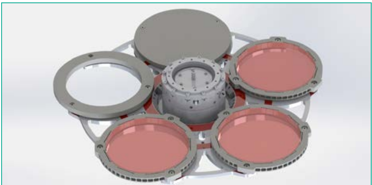
Fig. 1: The Filter Wheel Assembly (FWA) of the NISP Instrument. One can see the three filters, the open and closed position and the Cryomechanism installed in the center of the wheel.
