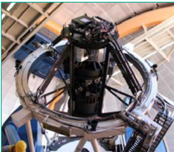
Fig. 1: The complete DES camera, DECam, installed at the prime focus of the Víctor M. Blanco 4-meter telescope at the Cerro Tololo Inter-American Observatory (CTIO) in the Chilean Andes.
