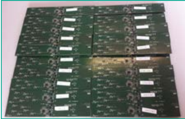
Fig. 3: Pre-production series of boards with the camera trigger functionality.
