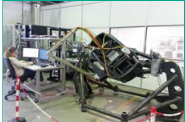
Fig. 2: The telescope simulator, with PAUCam mounted on it. The camera is open, and most of the elements are not installed inside.
