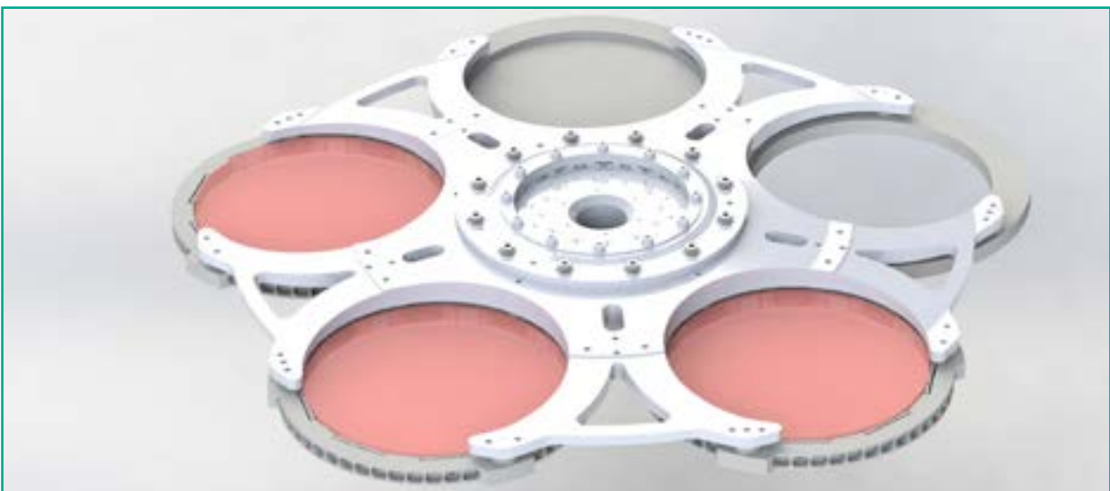
Fig. 3: The Filter Wheel Assembly (FWA) of the NISP Instrument. One can see the three filters, the open and closed position and the Cryomechanism installed in the center of the wheel.
