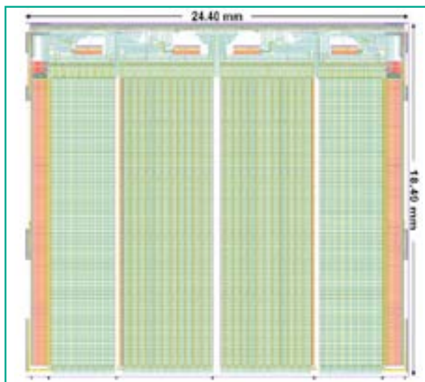
Fig. 4: The layout of the H35 demonstrator, fabricated in AMS 350 nm technology. The read out cell as well as other digital blocks have been designed by IFAE.
